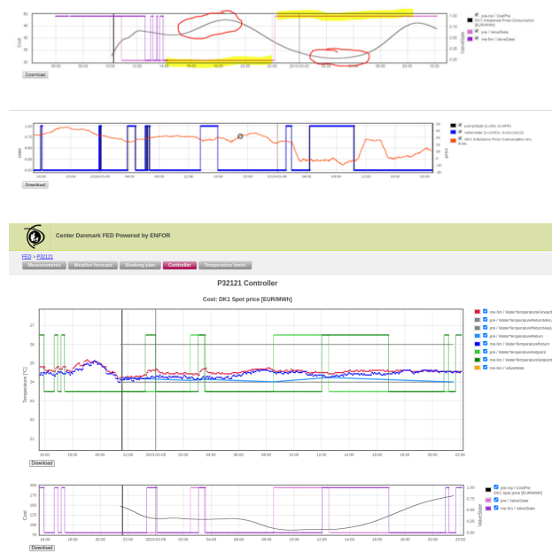
Figure 2 shows an example from the operation of the swimming pools in which the prices were negative. In this case the controller turned on heating until the temperature of the swimming pools reached their maximum allowed values.
